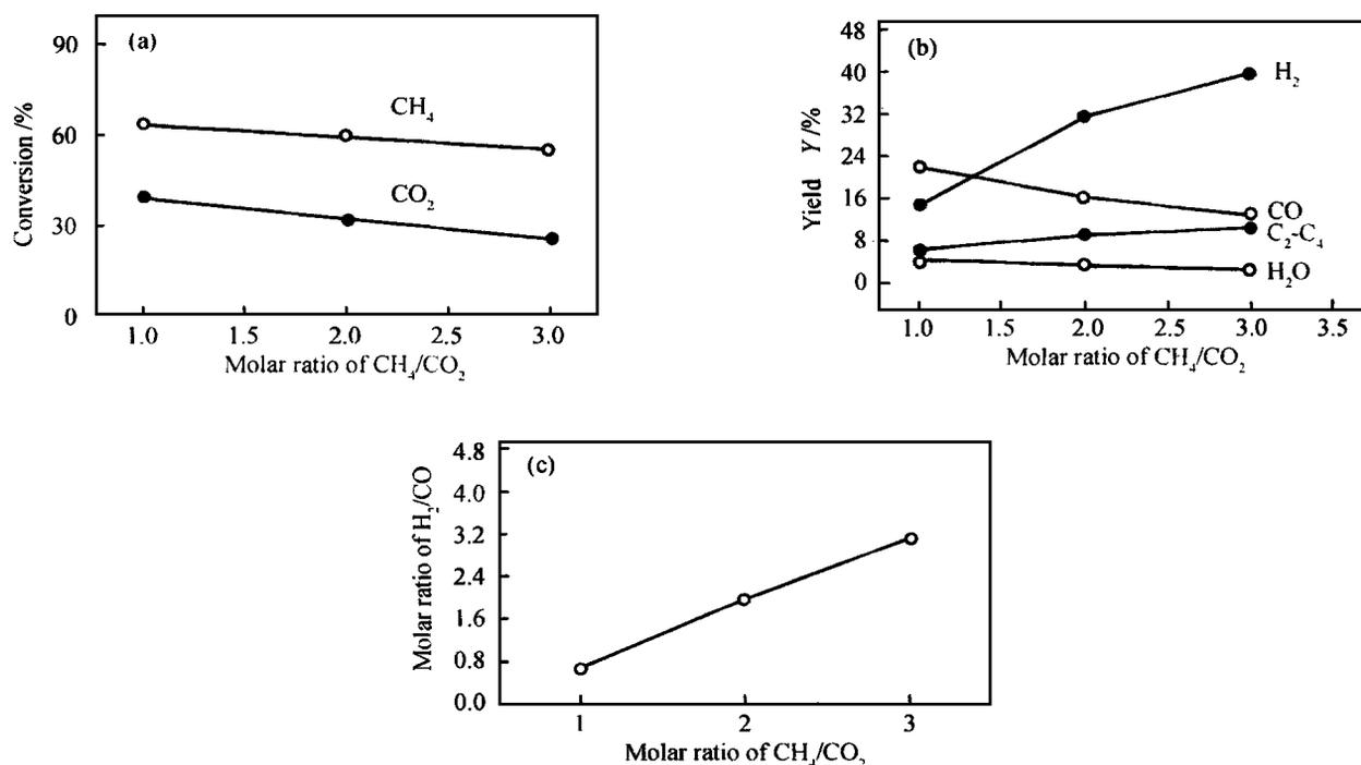
Figure 4 Effect of molar ratio of  $\text{CH}_4/\text{CO}_2$  on experimental results
