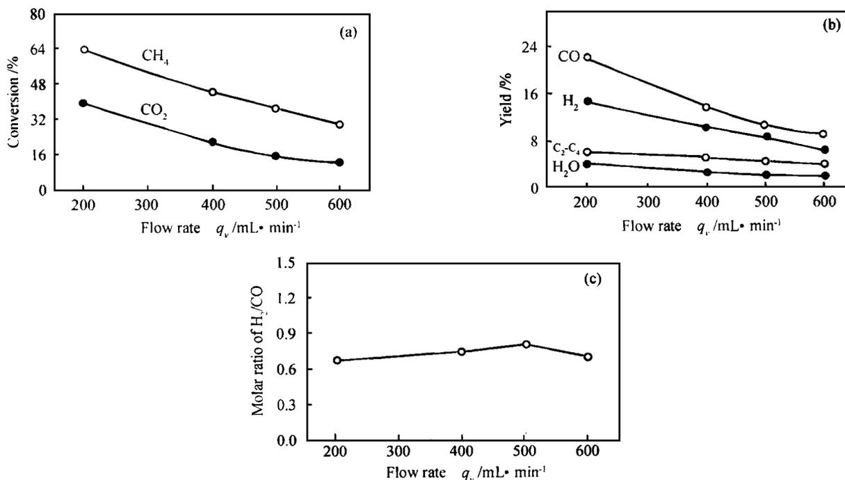
Figure 2 Effect of flow rate on experimental results
