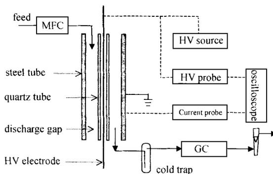
Figure 1 Configuration of DBD reactor and experimental setup
